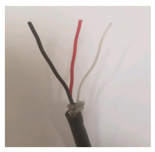
Prepare the Breezi cable as shown, cut the green wire and ground shield off.
