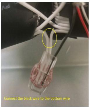
Not Included in the kit are the kit are (3) UR IDC connectors, (available from Home Depot). These are used to easily connect three wires together with a simple squeeze of plyers. Solder and shrink tube can also be used.
