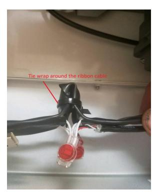
Make a 1 inch fold in the ribbon cable and secure with a tie wrap. Do not pinch the ribbon cable
