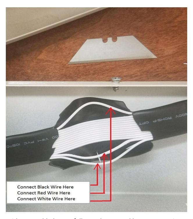
With a razor blade, carefully cut the top and bottom two wires from the ribbon cable as shown.
