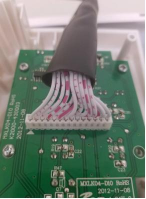
Locate the ribbon cable and cut the rubber sleeve as shown.
