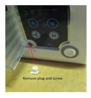
To remove the side panel and access the front panel control cable remove the rubber plug. Loosen the Philips screw and lay the unit face down on a protective surface. Remove the side cover by pulling up on the cover.
