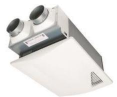
An ERV is an Energy Recovery Ventilator. They are similar to an HRV which is a heat recovery ventilator. HRVs and ERVs both supply fresh air to the home and exhaust stale air while recovering energy from the exhaust air in the process. The main difference between them is that an HRV transfers only heat while an ERV transfers both heat and moisture.
