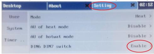
The switch status can be displayed in the C parameters
