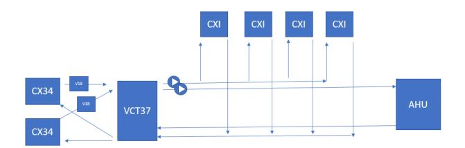
Below shows a basic drawing of something one of our customers did, shown here as an example of flexibility. In this example there is a 3-coil indirect tank with Chiltrix used for heating and/or cooling, and with two additional heat sources.
