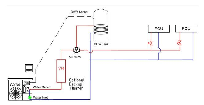
Note, no booster pump for DHW is shown above. This may be needed if you use a DHW tank with a small diameter coil or if the DHW tank is not close enough to the CX34. Otherwise, a booster pump is generally not needed for DHW.
