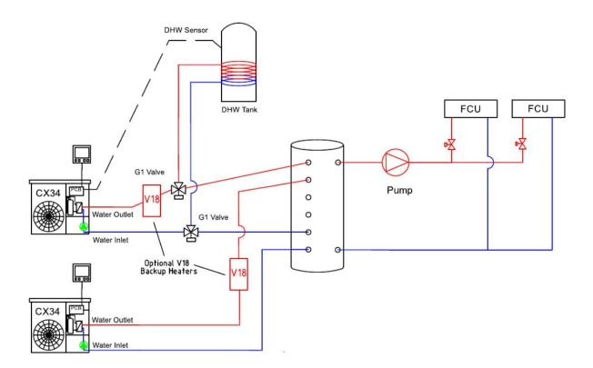
A hot water heating function is shown connected to one CX34. A loop pump (as shown above) is used on the load side of the buffer tank. 2x 3way valves are used with multiple CX34 when DHW is used.
