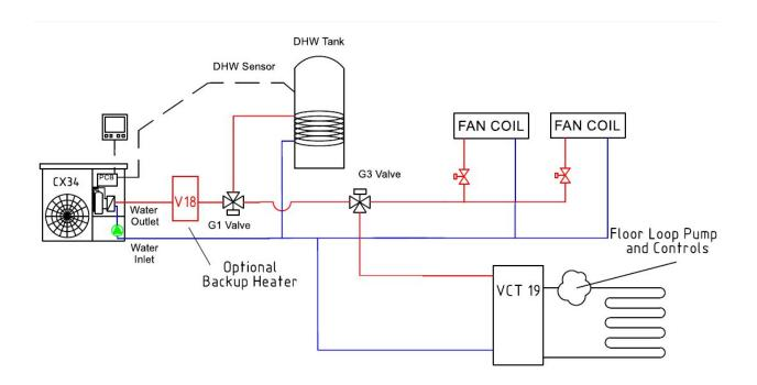
The above example is used when you want to isolate the heating (radiant) from cooling (fan coils). This also means that in this example, the fan coils would not be available for heating. For that reason, using the G3 seasonal valve design is not commonly used.
