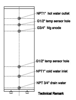
Ultra-High Grade Stainless Steel Duplex 2205 Inner Tank & Coil
