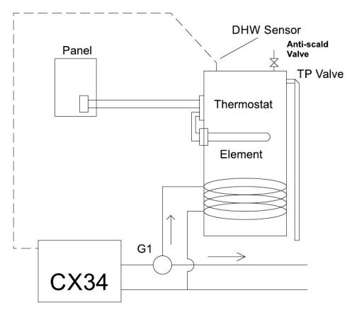
For anti-legionella, the Option #1 user will be required to manually set the tank tstat to 140F and hold it at that temperature for at least 6 hours, once per week, to prevent legionella growth. In this option #1, the backup electric element is always fully and solely controlled by the standard tstat set point.
