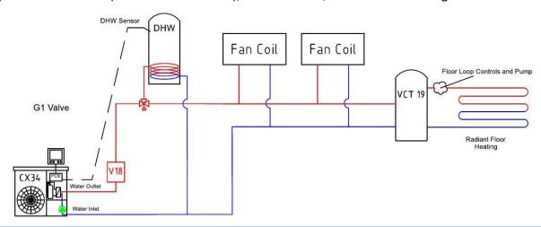
Prior to the introduction of the V18, Chiltrix provided backup heat in the same manner as all other leading brands, using an inline water heater (tank or tankless). However, these conventional approaches use a thermostat to target a water temperature resulting in temperature overshoot about 50% of the operating time.
