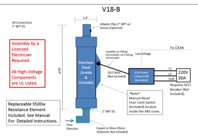
Must Be Mounted in Vertical Orientation
