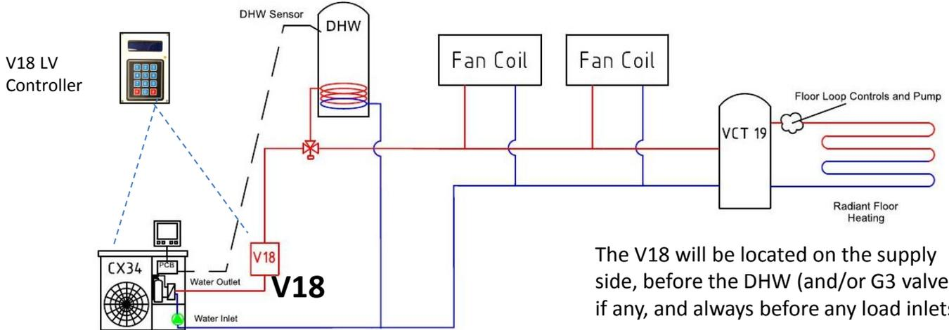
The V18 will be located on the supply side, before the DHW (and/or G3 valve), if any, and always before any load inlets.
