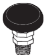
INSTALL VACUUM RELIEF IN COLD WATER INLET LINE AS REQUIRED BY LOCAL CODES.
