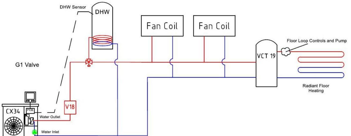
**Primary / secondary piping is not supported, when connecting to a floor heating loop always use a buffer tank. Buffer tanks are generally used only with floor heating.**
