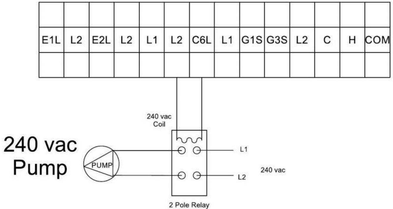
**When using a second NON-PWM water pump, use terminals L2 and C6L for relay coil power only. Do not connect a pump directly to L2 and C6L, always use a relay with a 240 vac coil. This pump will only run when the PWM pump is running. Setting P54=0 and P52=1, will shut C6 off when the chiller reaches its set point.**
