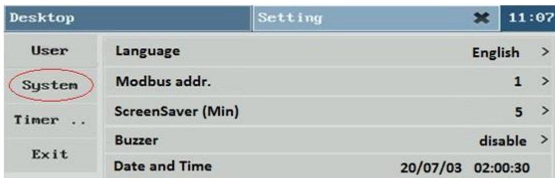
The Modbus address can be changed by touching “System”, then Modbus addr.
