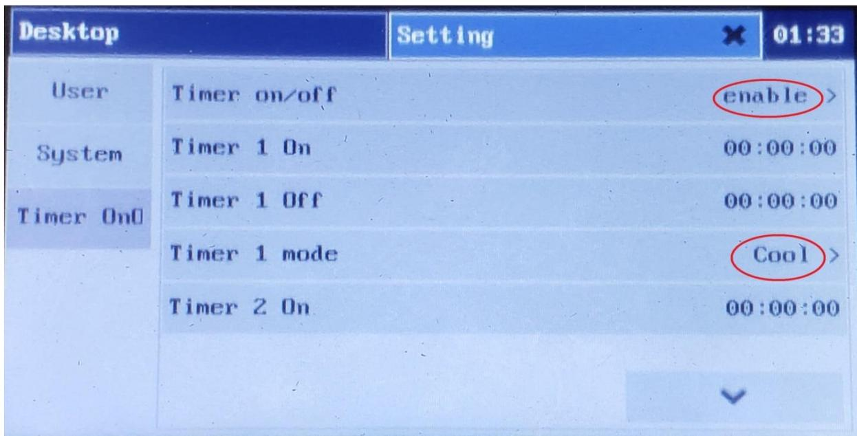
To use the timer functions the timer on/off must be enabled. There are 4 timers labeled timer 1-4 with a mode selection for each timer.
