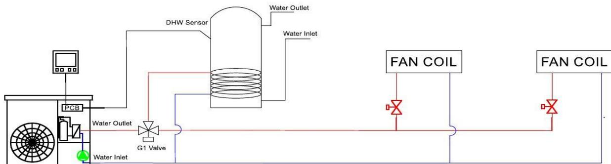
DHW target setting temperature is the tank water temperature measured with the DHW sensor, not the inlet water temperature. If the target temperature is 122°F, (refer to page 43 to set the DHW temp), and the differential is 2°C, it means, when the DHW tank reaches 122°F, the compressor will stop. When the DHW tank temperature is lower than 119°F, the compressor will start.
