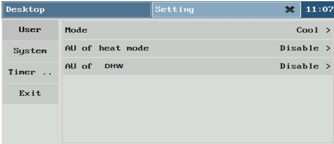
Touch the mode bar and the screen below will appear. Select the mode you want by touching the bar associated with the mode. AU Heat Mode and AU DHW Modes are not used on the CX34 and should be disabled.
