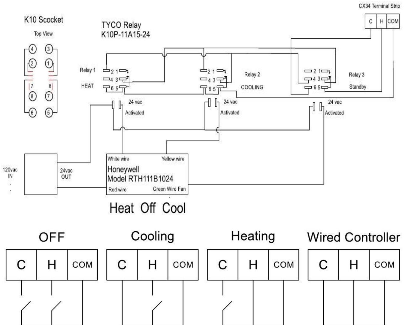
Once the relays are wired as shown the CX34 DIN setting must be changed
