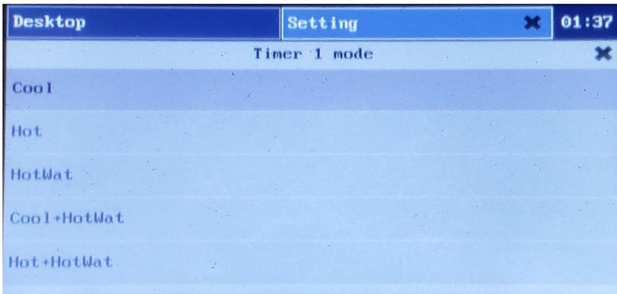
There are 5 modes that can be set to use electricity when the rate is lower. Only one mode can be set for each timer 1-4.
