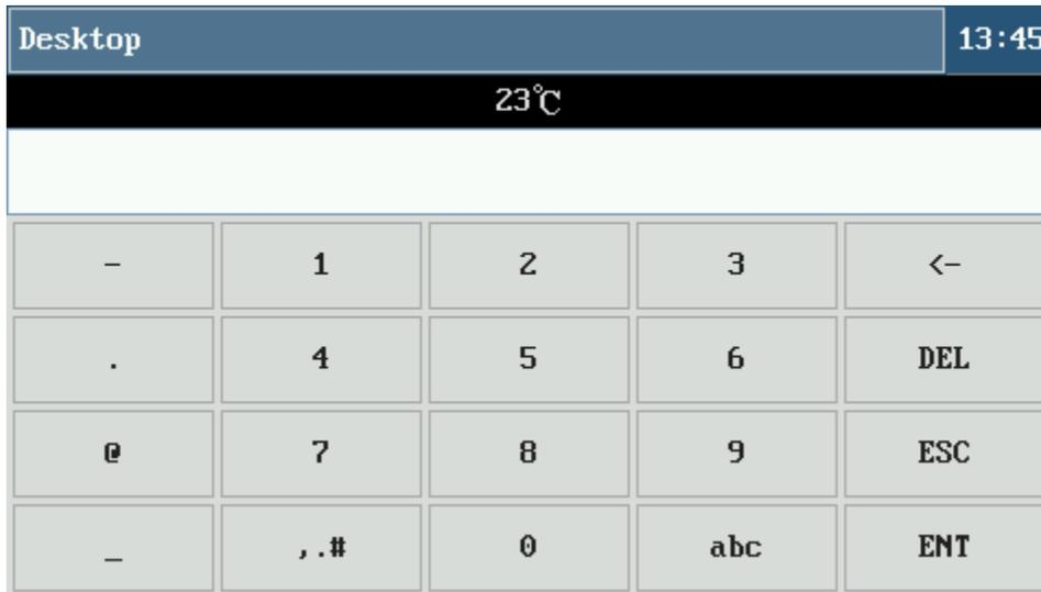
Next, to set the temperature, go back to the desktop and touch the “set target AC” icon. Using the keypad select the desired temperature and touch the “ENT” icon.
