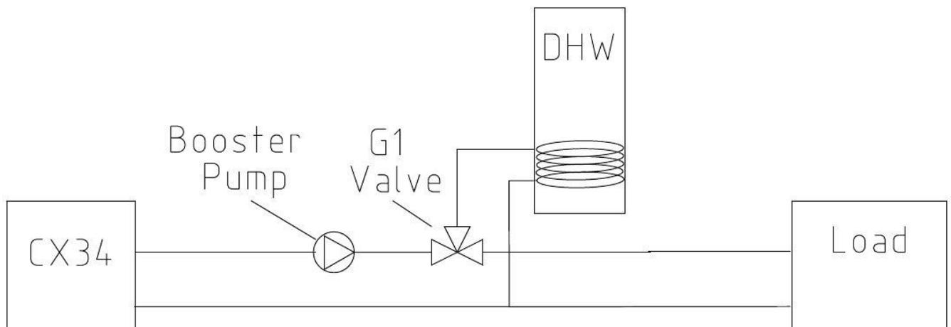
A booster pump may be installed in front of the G1 valve when installing the DHW option if the distance between the G1 valve and DHW tank exceeds 25 feet.
