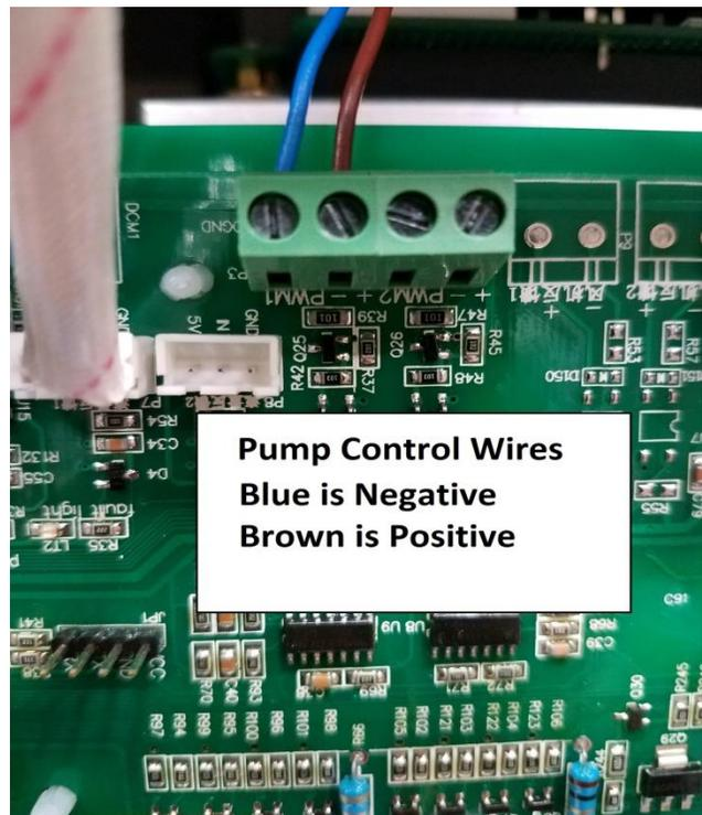
The blue and brown pump **CONTROL WIRES** are connected to the (+ & -) on the PWM1 terminal connector at the top or the main control pcb.
