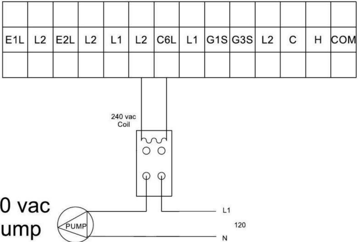
Connect the fixed speed pump to L2 and C6L.
