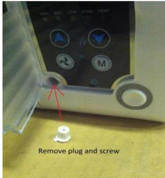
To remove the side panel and access the front panel control cable remove the rubber plug. Loosen the Philips screw and lay the unit face down on a protective surface. Remove the side cover by pulling up on the cover.
