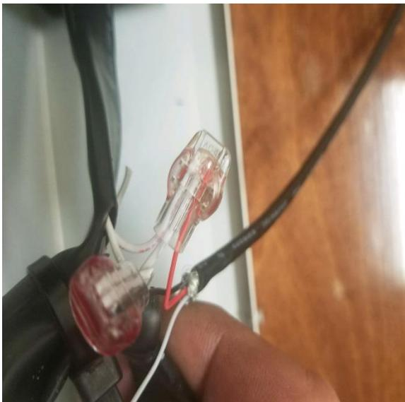
The red wire is connected to the second from the bottom of the ribbon cable with a UR IDC connector.
