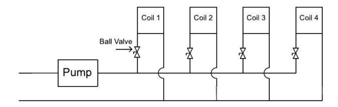
Close the input valve to each fan coil except the last coil (4). Turn the pump on and run it, when the bubbles stop coming out of the discharge hose turn on the ball valve on coil (1), wait for the bubbles to stop, then do the same for coil number (2), then (3). All CX Chillers are required to have a flow switch installed in the loop. Air in the system may cause a flow switch alarm; the controller will display a P5 or P6 error code.
