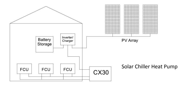
Standard PV panels should be sized to match the maximum daily energy needs of running the chiller. When solar power exceeds the needs of the chiller, extra power is sent to the batteries. When solar power is less than chiller requirements, or at night, power is pulled from the batteries as needed. Solar array and batteries must be properly sized based on location and duty cycle.
