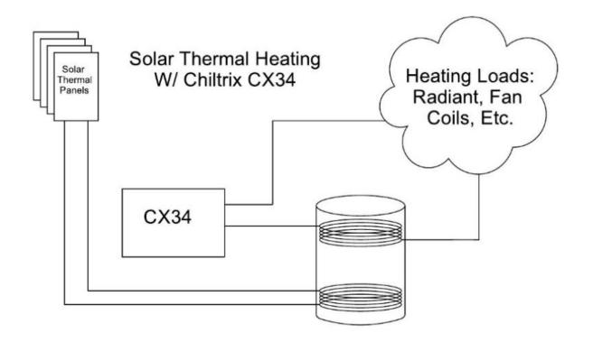
Above shows an atmospheric tank with two coils. Single coil designs and various tank options are also possible.
