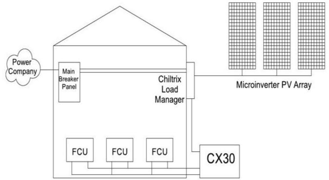
Microinverter PV should be sized to match the expected annual energy needs of running the chiller for heating and cooling. Larger systems can use a string inverter in a similar manner. When solar power exceeds the needs of the chiller, extra power is sent to other electrical loads. When solar power is less than chiller requirements, additional power is pulled from the grid. If solar power exceeds all loads, excess is sent to the power grid for a credit to be used later, requires net-metering.
