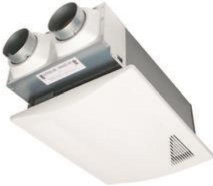
An ERV is an Energy Recovery Ventilator. They are similar to an HRV which is a heat recovery ventilator. HRVs and ERVs both supply fresh air to the home and exhaust stale air while recovering energy from the exhaust air in the process. The main difference between them is that an HRV transfers only heat while an ERV transfers both heat and moisture.
