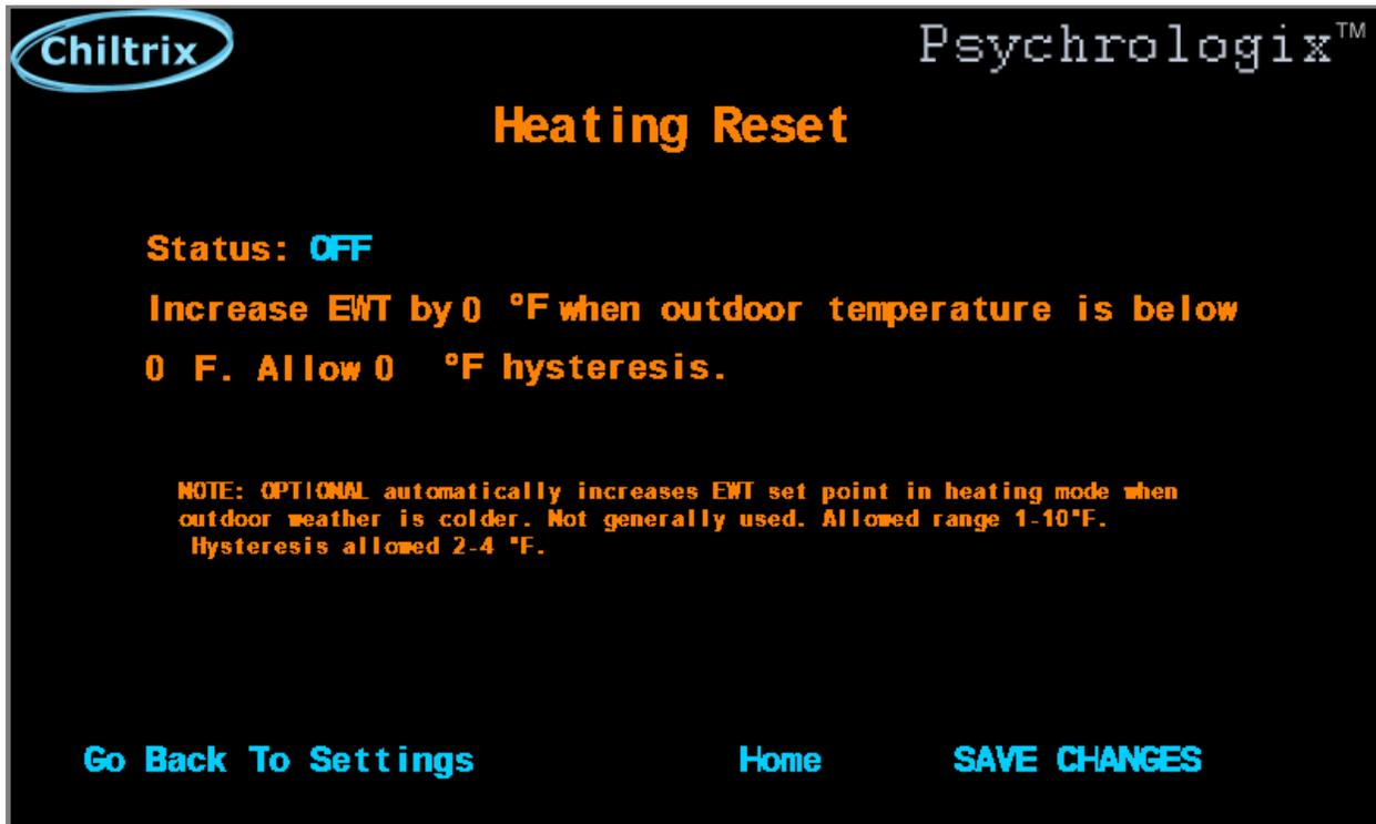
If your CX34 has onboard dynamic reset, do not use this feature in the Psychrologix unless using a 3<sup>rd</sup> part backup that starts at a specific outdoor temperature. For most normal applications, there is a more full-featured and more capable version onboard all CX versions since 2019.
