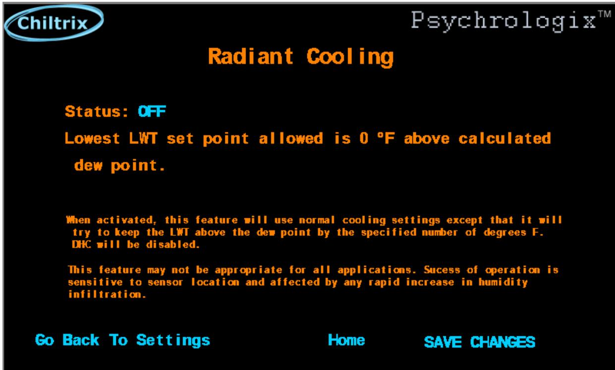
If you wish to provide radiant cooling, it must not produce condensation (does not de-humidify) you may be interested in this feature. Condensation can produce water in places where you do not want it, radiant cooling therefore requires that the loop temperature be above the dew point. The design is intended to keep the cooling loop as cool as possible while remaining above the dew point as a priority. Buffer tank(s), system size, and associated thermal lag, will affect how well this works.
