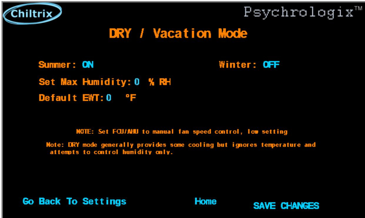
This mode is manually activated from the main screen when needed. Only “summer” or “winter” can be set at a time, not both. These settings allow for a large energy savings for an un-occupied building. In summer, a setting of Max Humidity will allow humidity to be controlled without regard to temperature, and in winter, to prevent interior space freeze damage with the minimum amount of energy usage.
