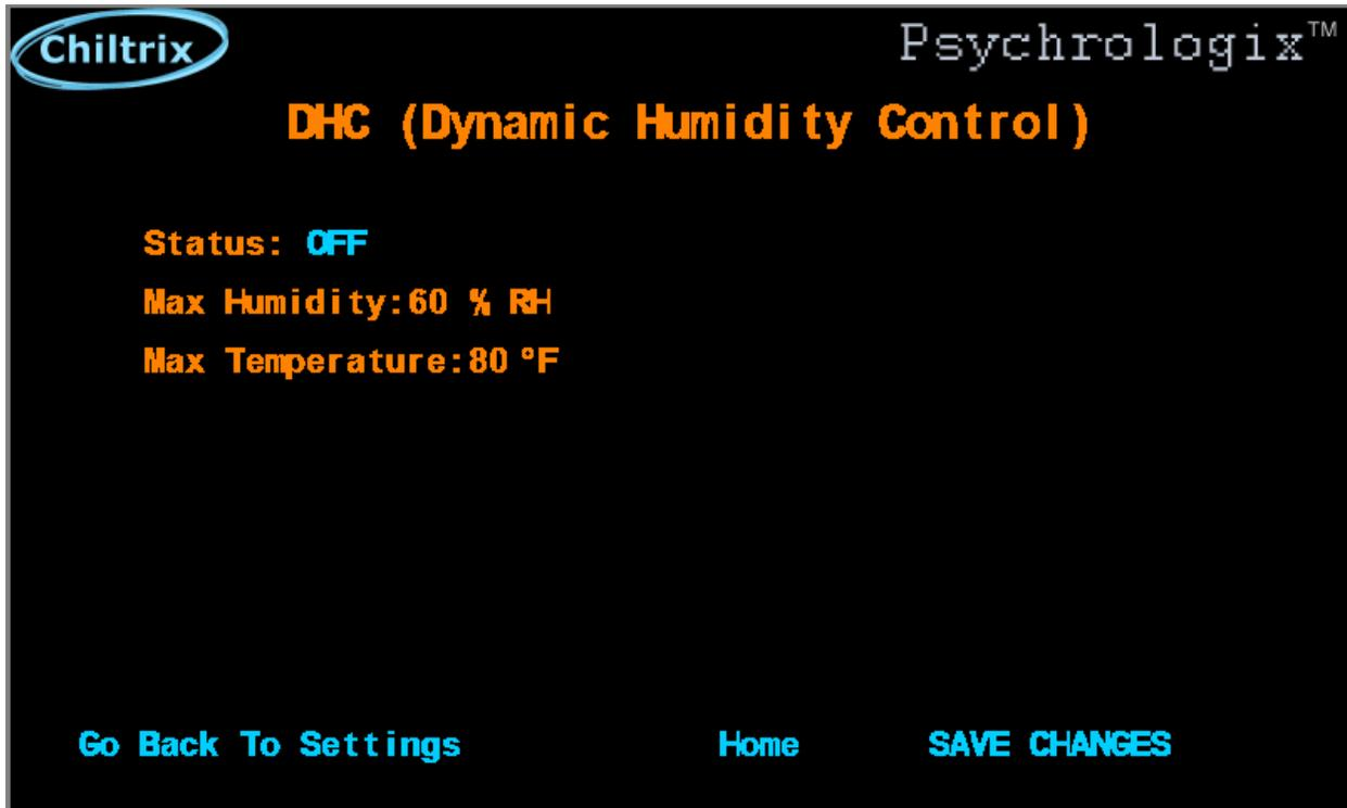
For many users, this is the most important feature of the controller as it can tightly control humidity, prevent over-dehumidification, and save a large amount of energy.
