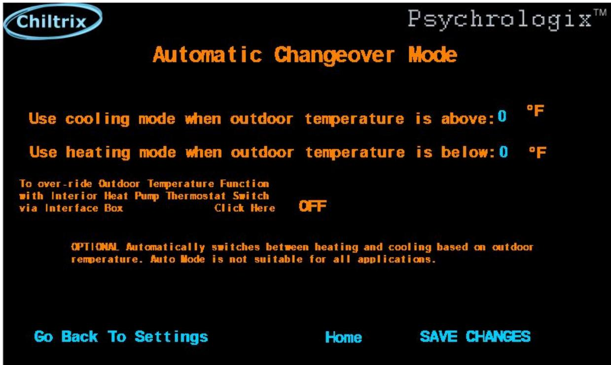
If your CX34 has automatic switchover mode onboard, do not use this feature in the Psychrologix. There is a more full-featured and more capable version onboard all CX34 versions since 2021 (Use this only for CX34-1, CX34-2, CX34-3)
