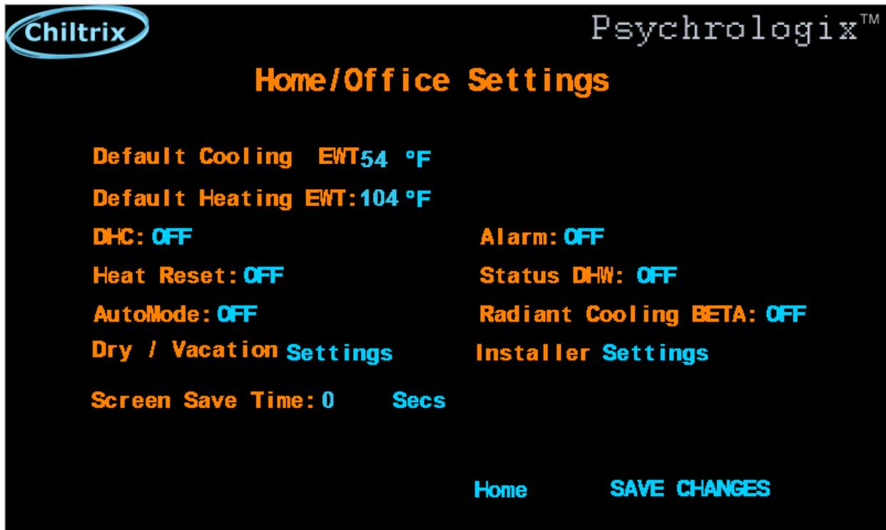
The settings you recorded from the standard controller can be input on this and subsequent screens, as applicable. Tap items in blue to change settings, when finished touch “SAVE CHANGES”.
