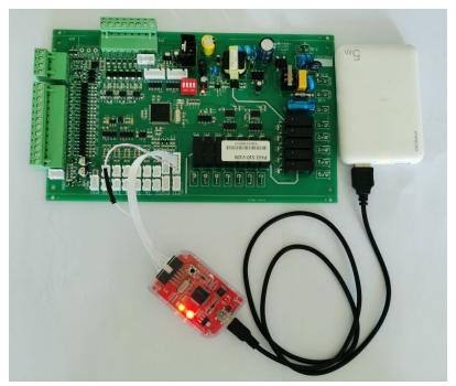
6. Press the black button to program the board and the programmer will light up orange and red.
