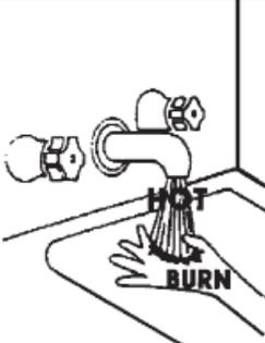
Water temperature over 125°F (52°C) can cause severe burns instantly resulting in severe injury or death.
