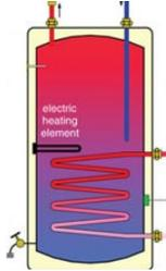
This type of tank should have at least one backup heating element/thermostat, magnesium anode, TPV (temperature/pressure valve), and an anti-scald valve installed on the hot water outlet. The backup element may be fully controlled by the element tstat. Power to the element/tstat may or may not be controlled by Chiltrix depending on system design. An anti-legionella (automated or manual) function must be employed, see section on legionella.
