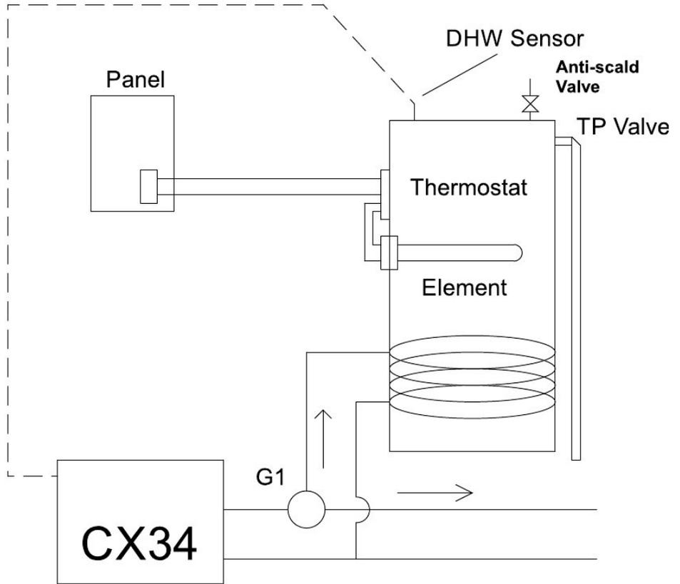
**For anti-legionella, the Option #1 user will be required to manually set the tank tstat to 140F and hold it at that temperature for at least 6 hours, once per week, to prevent legionella growth. In this option #1, the backup electric element is always fully and solely controlled by the standard tstat set point.**
