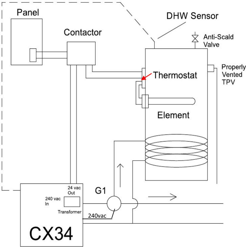
In Option 2, the CX34 controls the tank temperature. The element thermostat is set for 140F, which only controls the upper limit. Actual tank temperature setting and element is controlled by the CX34.
