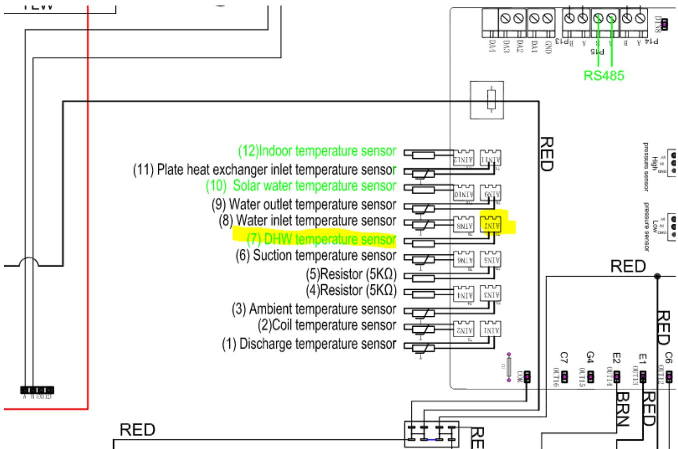
To enable DHW a DN25(G1) valve must be installed and enabled. For dual CX34s there will be 2x DN25 valves wired in parallel. DHW is enabled from the standard controller as: HotWater, Cooling & HotWater, or Heating & HotWater.
