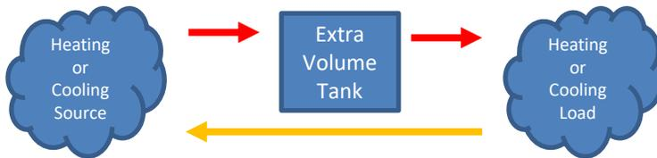
While not recommended, backup heat can be installed inside an inline volume expander tank. In this case a tank thermostat and TPV must be installed. Contact Chiltrix technical support for instructions. The recommended backup solution is the optional V18 dynamic variable backup heater.
