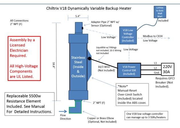
Must Be Mounted in Vertical Orientation
