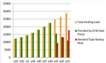
Shown above left, the V18 targets a precise match to the BTU shortfall based on real time information from the CX34. Right side chart shows a standard thermostat controlled backup heater. The V18 allows the compressor to provide a higher percentage of the total heat, improving the average COP of the system. Shown with optional sensor adapter, not generally needed.
