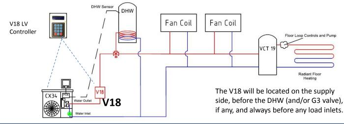
Prior to the introduction of the V18, Chiltrix provided backup heat in the same manner as all other leading brands, using an inline water heater (tank or tankless). However, these conventional approaches use a thermostat to target a water temperature resulting in temperature overshoot about 50% of the operating time.
