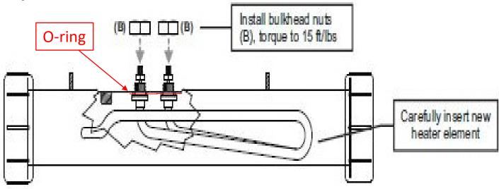
Visually inspect the element after installation and verify that that the element is not in contact with the inside wall of the heater body. Failure to do so may cause failure.
