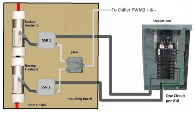
Two (or three) V18 inline heaters may be mounted together (series piping), note they are wired separately for power, each with a 30a GFCI circuit for main power. Control circuits are wired in parallel and the CX Unit controller can manage up to 3x V18 units. Shown below, two V18Bs piped in series.
