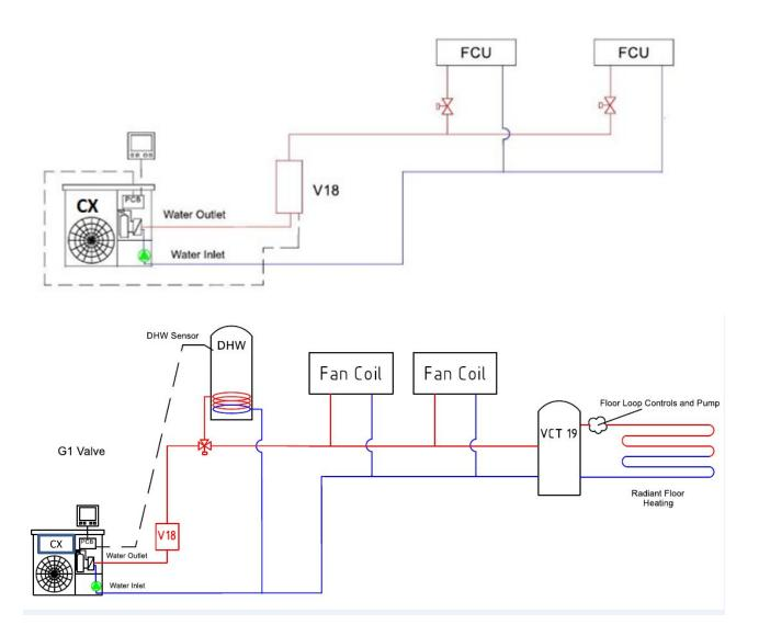
The V18 must be installed in an upright orientation (vertical) and the water flow entry should be from the bottom. The bottom, or water entry end, is considered to be the end closest to the removable panel as shown in all pictures.
