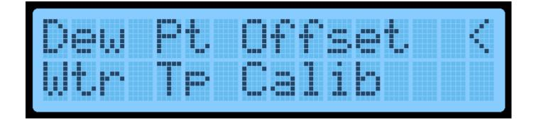
The dew point offset is a target in relationship to the dew point. Example: if the offset is +4F and the highest dew point read from the sensors is 54F then the controller will target an output temp of 58F. If the setting is -4F and the sensors are reporting a dew point of 54F then the target would be 50F.
