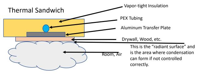
Above, "thermal sandwich" shown as ceiling radiant. For floor radiant, just turn it upside down.
