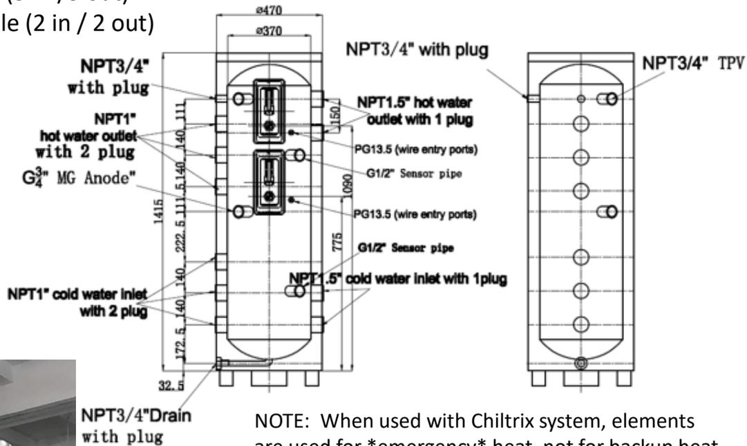
NOTE: When used with Chiltrix system, elements are used for \*emergency\* heat, not for backup heat. For backup heat, see Chiltrix V18.
